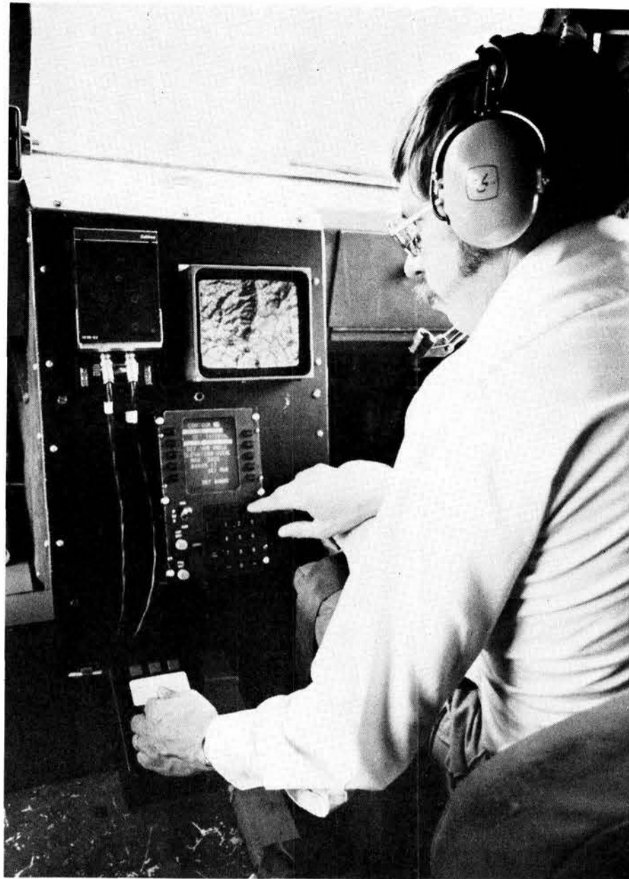
ED NAVA (5343) makes final adjustments on a terrain-aided navigation system in an experimental multi-purpose Army vehicle before a field test. The unique system uses computer-generated color maps, displayed on a dashboard screen, as a means of giving operators a continuous fix on vehicle location. A similar system will be tested in a military jet later this year.
